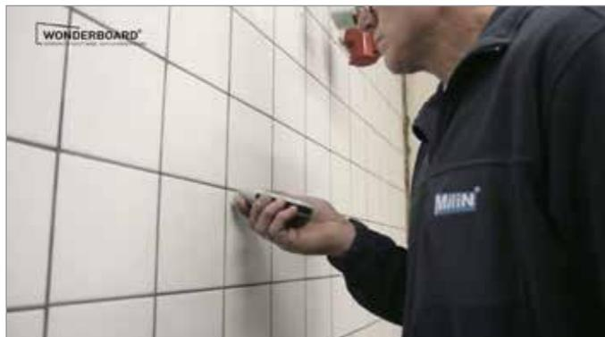
The moisture content in the wall can be measured using a moisture meter.
