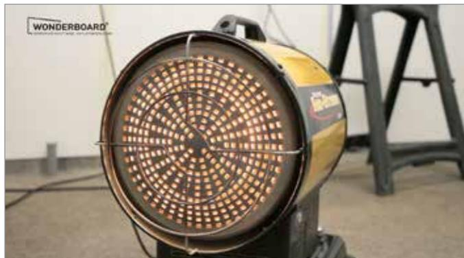
The walls must be dry, not just visually, but the actual moisture must be removed from within the wall. This can be achieved by installing a building dryer in the relevant space for a considerable time or by setting the heater to high. The duration will depend on the condition of the walls.
